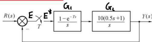
解: 设  $G(s) = \frac{10(0.5s+1)}{s^2}$ , 由  $E(z) = R(z) - G_1 G_2(z) E(z), Y(z) = G_1 G_2(z) E(z)$  知
