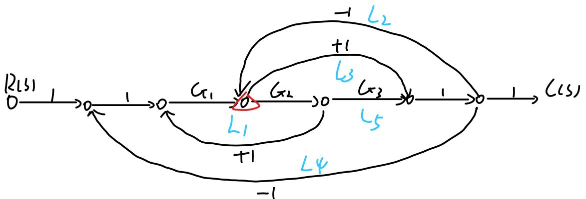
$$\text{回路} \cdot L_1 = G_1 G_{11}, L_2 = -1, L_3 = -G_2 G_3, L_4 = -G_1 G_2 G_3, L_5 = -G_1,$$
