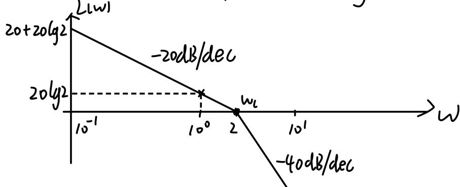
$$\text{计算 } \omega_c: -20 = \frac{0 - 20 \lg 2}{\lg \omega_c - \lg 10^0} \Rightarrow \omega_c = 2 \text{ rad/s, 恰好在转折频率处}$$
