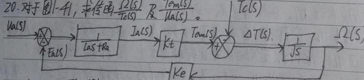
令  $T_0 = 0$  求  $\frac{T_e(s)}{U_a(s)} = \frac{K_t I_a(s)}{E_a(s) + I_a(s)(R_a + Ls)}$
