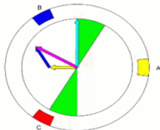
BLDC Six-Sector Commutation Two Pole-Pair
