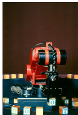
Figure 1.67: H. Asada and T. Kanade at CMU (1981): Direct drive robots
