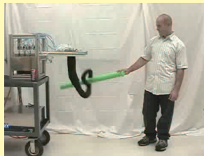
Figure 3.22: OCTARM, a hyperredundant (continuum) manipulator with 27 DoF
