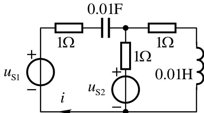
图示电路容抗  $X_C = -\frac{1}{\omega C} = -\frac{1}{100 \times 0.01} \Omega = -1 \Omega$ ,
