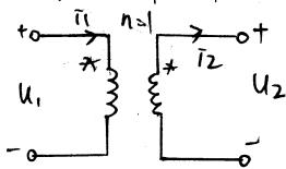
$$\left. \begin{array}{l} U_1 = n U_2 \\ i = \frac{1}{n} i_2 \end{array} \right\} \quad \text{若} i_1 \uparrow \text{时, 互感磁通增大, 则另一端电流} \\ \text{从} i_2 \text{流出以抵消互感电势} \rightarrow i_2 \text{也增,} \\ \text{(非同名端流入)} \quad i_1, i_2 \text{同向减, 方向正确.}$$
