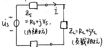
$$\text{回路电流 } \dot{I} = \frac{U_s}{\sqrt{(R_s + R_L)^2 + (X_s + X_L)^2}}$$
