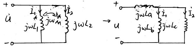
$$\text{其中 } L_a = M, \quad L_b = L_1 - M, \quad L_c = L_2 - M.$$
