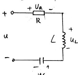
$$\begin{aligned} u &= u_R + u_L + u_C & u_R &= RI & u_L &= j\omega L I & u_C &= \frac{1}{j\omega C} I \\ && \Rightarrow u &= [R + j(\omega L - \frac{1}{\omega C})] I & &= j X_L I & &= j X_C I \\ && & & & & \rightarrow \text{阻抗模.} & \\ && & & & & & z = R + j(X_L + X_C) = R + jX = |z| \angle \varphi \rightarrow \text{阻抗角 (因为 } \varphi \text{ 与 } \psi \text{ 相同)} \end{aligned}$$
