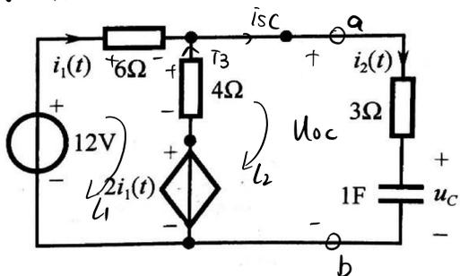
① 求开路电压 由  $l_1$  KVL:  $6\bar{i}_1 + 4\bar{i}_1 + 2\bar{i}_1 = 12$
