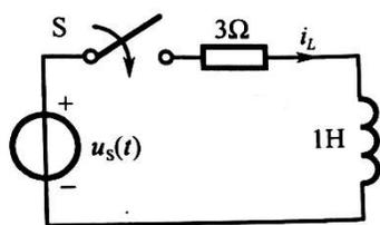
$$u_s(t) = 10\sin(4t + \theta) = 10\cos(4t + \theta - 90^\circ) \quad \text{接入角为 } \psi_u = \theta - 90^\circ$$
