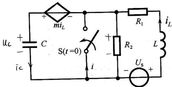
解: 换路前,  $i_L = \frac{U_S}{R_1+R_2} = 2A$      $U_C = m i_L + R_2 i_L = 16V$
