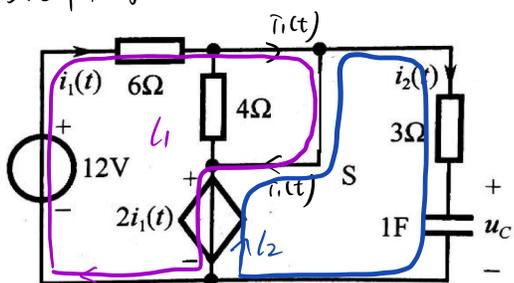
由回路  $l_1$  KVL  $6\bar{i}_1 + 2\bar{i}_1 = 12 \Rightarrow \bar{i}_1 = \frac{3}{2}A$
