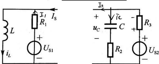
左支电路:  $T_1 = \frac{L}{R_1} = 0.4s$
