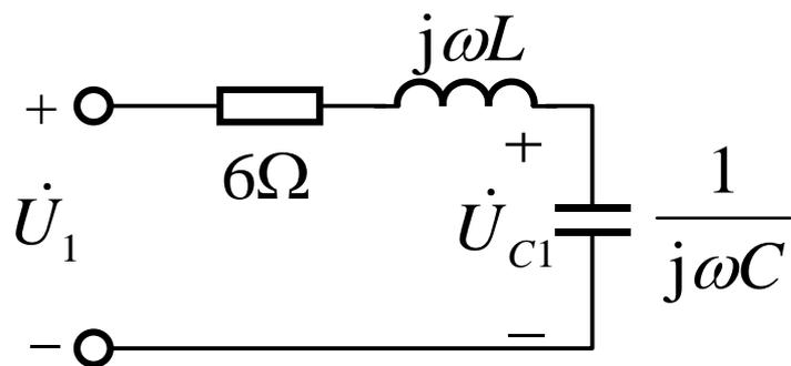
$$\begin{aligned} \dot{U}_{C1} &= \frac{\frac{1}{j\omega C}}{6 + j\omega L + \frac{1}{j\omega C}} \dot{U}_1 \\ &= \frac{-8j}{6 + 2j - 8j} 12\angle 0^\circ = \frac{16}{\sqrt{2}} \angle -45^\circ V \end{aligned}$$
