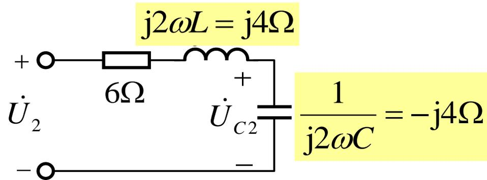
$$\begin{aligned} \dot{U}_{c2} &= \frac{\frac{1}{j2\omega C}}{6 + j2\omega L + \frac{1}{j2\omega C}} \dot{U}_2 \\ &= \frac{-4j}{6 + 4j - 4j} 6\angle 0^\circ = 4\angle -90^\circ \text{V} \end{aligned}$$
